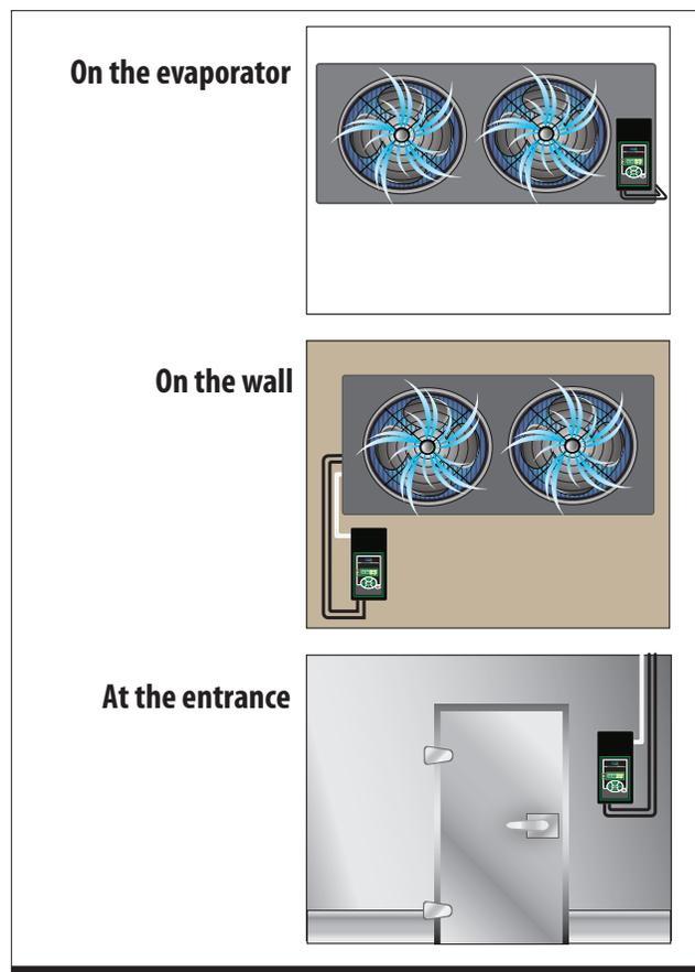
Although there is one pressure transducer and four temperature sensor inputs, when used with mechanical valves (TEVs), KE2 Evap only requires the **(2) sensors supplied with the kit**. One sensor reads the return air temperature and the other measures the coil temperature. **NOTE! Sensor location is critical to the proper operation of the controller.**
