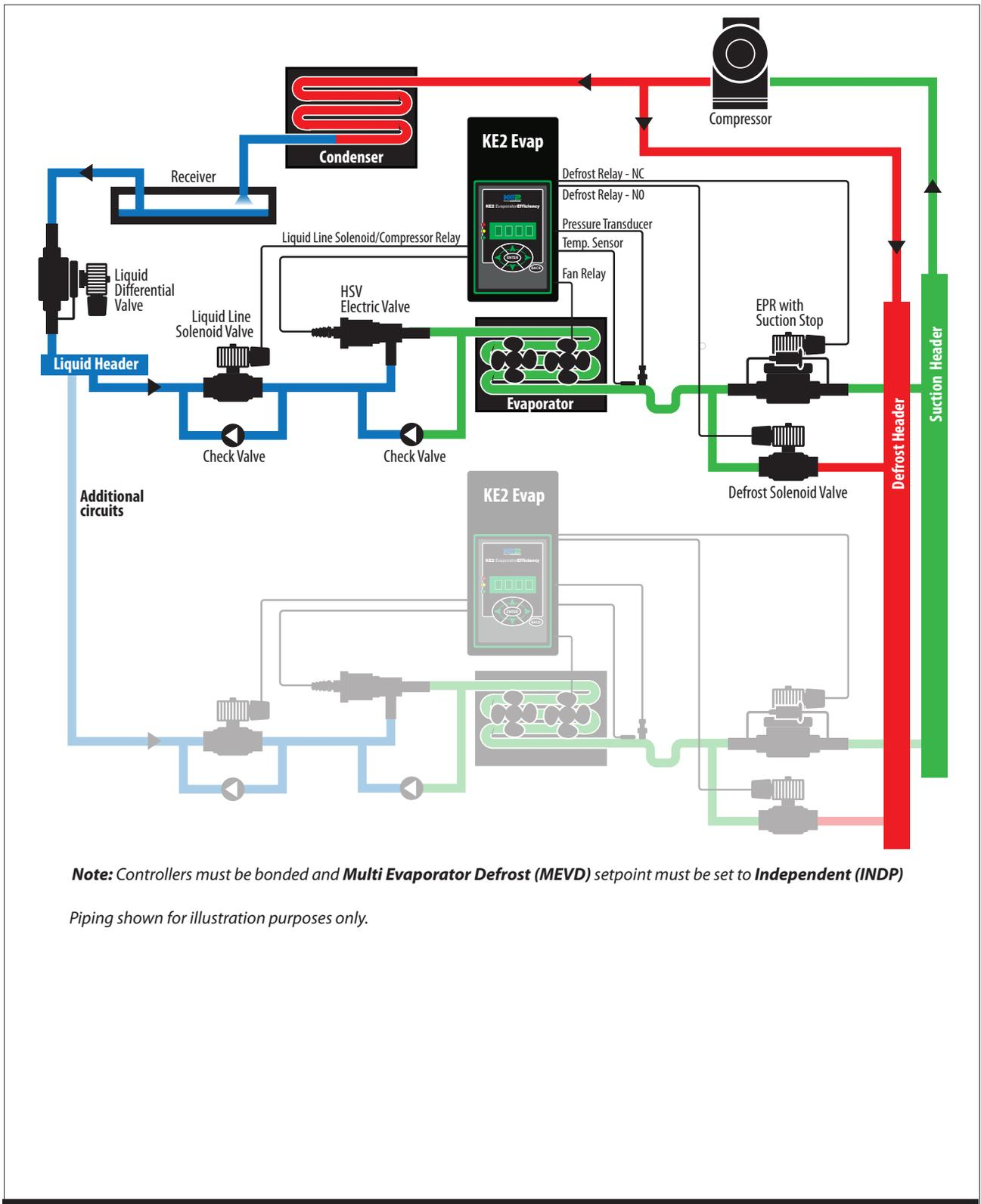
**Note:** Controllers must be bonded and **Multi Evaporator Defrost (MEVD)** setpoint must be set to **Independent (INDP)**
